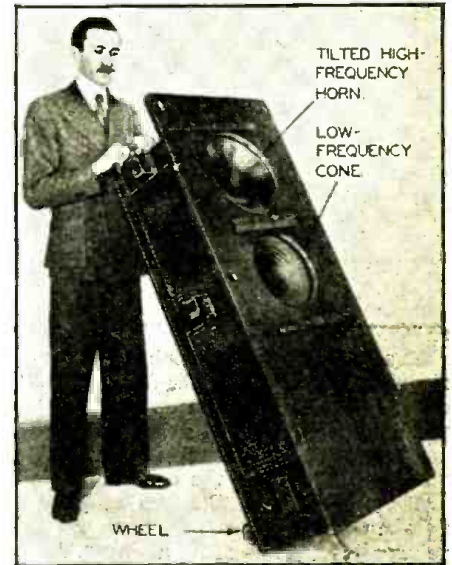
Fig. E. The amplifier and dual-speaker unit for the reproduction of high-fidelity wired sound. Wheels and a handle permit easy transportation.
