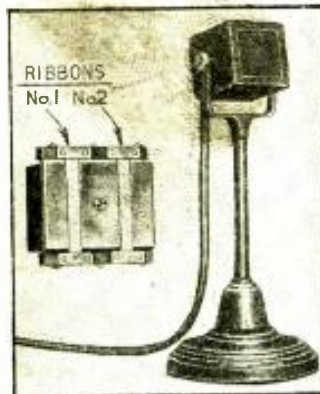
A double-ribbon microphone. (1075)
